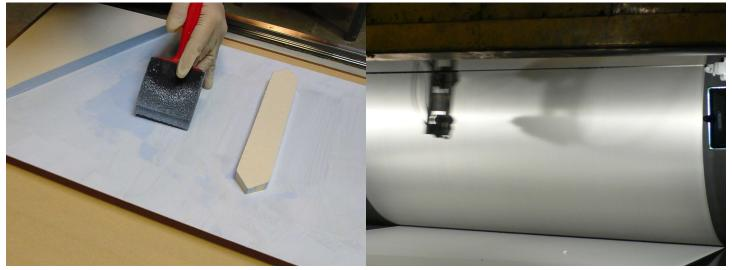
**SLICOAT-ES** is a very stable suspension of Boron Nitride crystals in water. These crystals make up 80+% of SLICOAT-ES's solids, making this paint-like coating an extremely effective non wetting coating for use on castertips, headboxes, launders and other melt contact surfaces.
