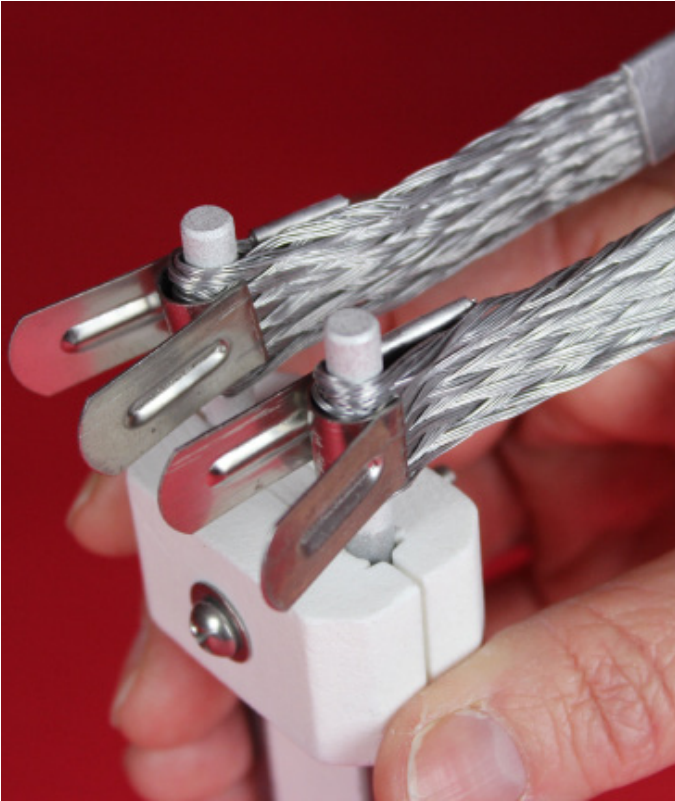
50-Amp straps are connected to MoSi 2 Element terminals with the use of a Manual Terminal Clamp Type MTC.
