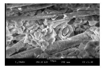
This image shows AL-28/1800's compositized microstructure in which its high-purity filler is tightly sintered in place and its  $AI_2O_3$  fiber is held in a strong mullite-composite binder.
