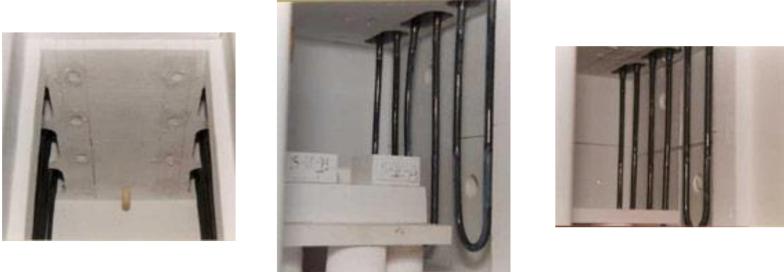
Fig. 6. An 1800 °C furnace is shown prior to the first firing (left). The chamber is 229 mm wide by 254 mm deep by 203 mm high. The volume is 11.8 L (0.4 ft 3 ). After 1 h of soak at 1800°C, the heating elements become distorted (center). After five cycles, with the fifth at a 24-h hold, the insulation shows minimal degradation (right). (See Fig. 8.)
