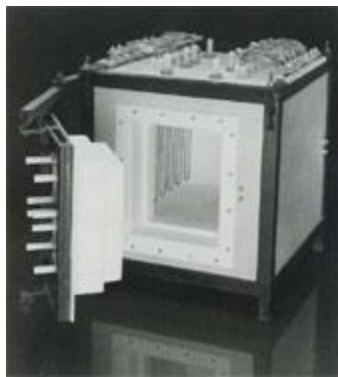
Fig. 4. A 1750° C furnace typically has a chamber 254 mm wide by 280 mm deep by 229 mm high. The typical firing schedule for this type of furnace shows that the element watt loading is critical for optimum performance.
